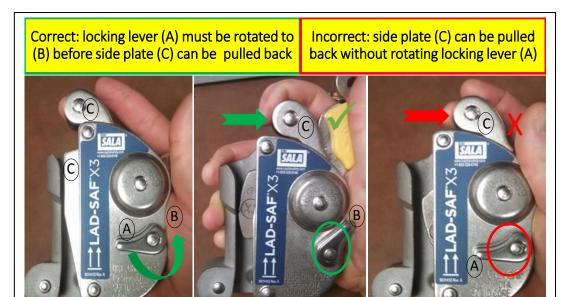
Proper operation of the sleeve is shown in green above. The locking lever (A) must be rotated to position (B) for the side plate (C) to be pulled backwards. If your sleeve functions in this manner, it is working properly. If you are able to pull the side plate (C) back by pulling on the top roller without first rotating lever (A) to position (B), then the unit should be removed from service (see red example above).
